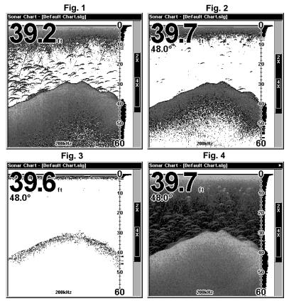
These figures show different sensitivity levels at same location. Fig. 1: Sensitivity at 88 percent, determined by Auto Sensitivity. Typical of full auto mode. Fig. 2: Sensitivity set at 75 percent. Fig. 3: Sensitivity set at 50 percent. Fig. 4: Sensitivity set at 100 percent.
